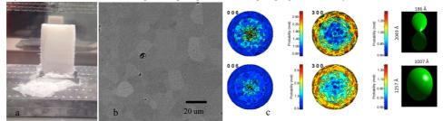
Figure 1. Growing alumina monolith in the climate chamber (a), backscattered electron image of the sintered ceramic (b) and pole figures with crystallite shapes from the XRD texture analysis (c).
