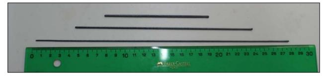
Figure 1:  $Bi_2Ca_2Co_{1.7}O_x$  grown rods depending of their initial green shapes before the translating growth (50 mm/h).
