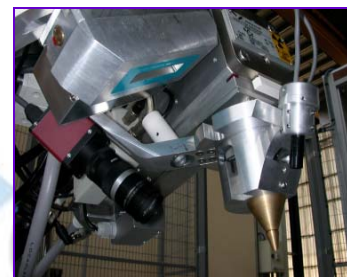
Head of analysis A compact diffraction device, combined with optical metrology
