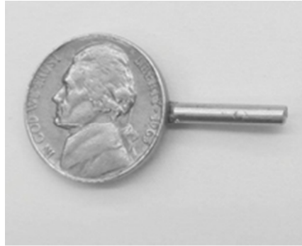
Figure 2. Typical sample for a hard X-ray diffraction experiment: Nickel coin mounted on a pin. 17x14mm (300 x 300 DPI)
