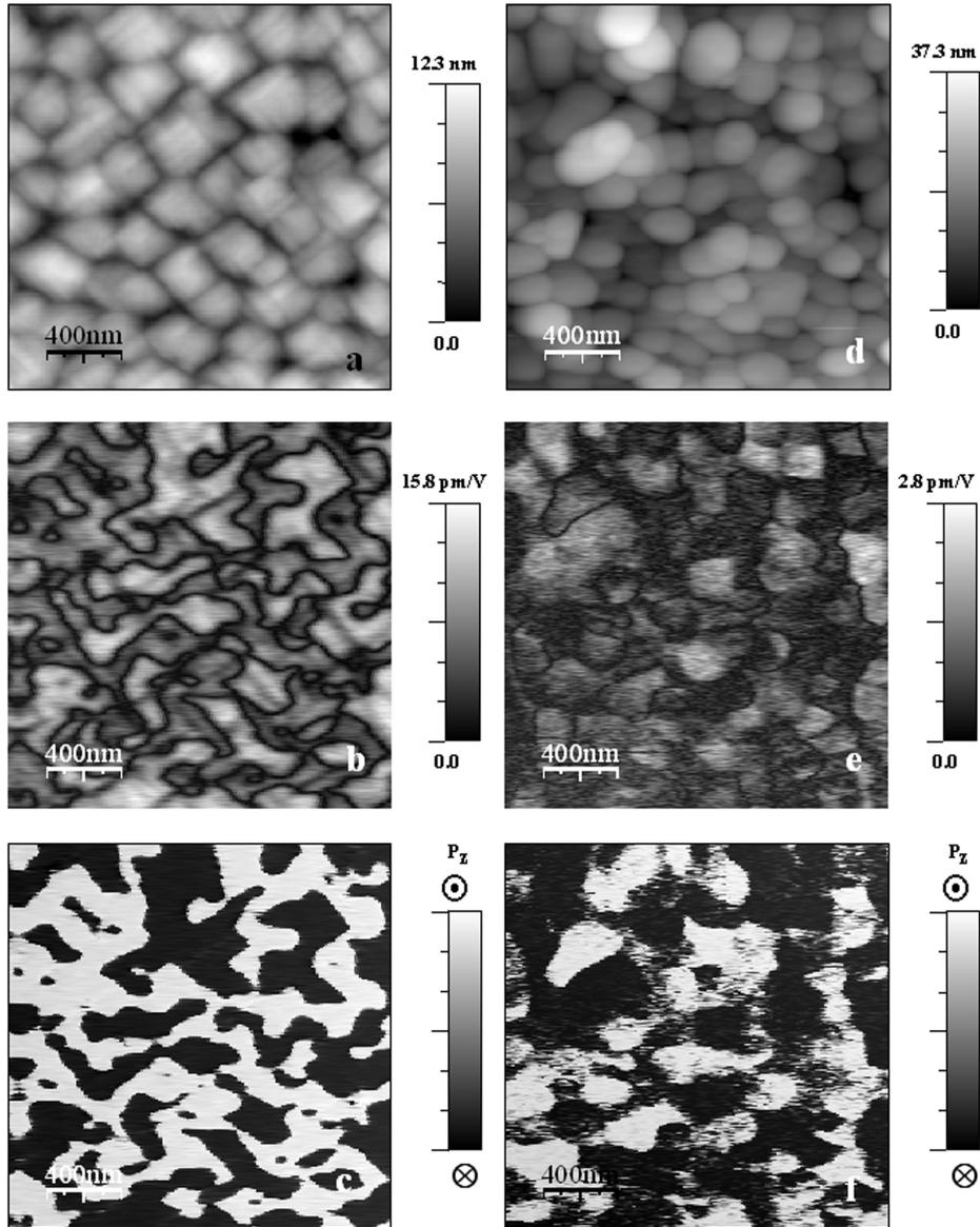
**Figure 4.** SFM images of PZT films deposited on an MgO (a–c) and on a Si-based substrate (d–e). Top to bottom: topography, piezoresponse amplitude and piezoresponse phase.
