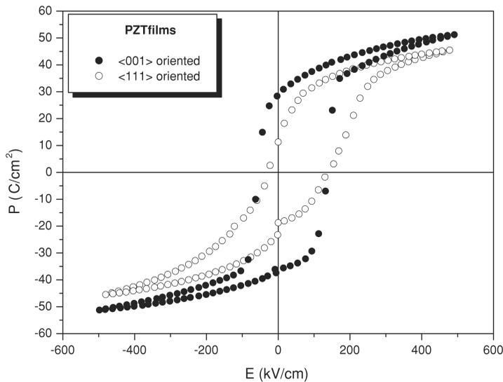
**Figure 3.** P-E hysteresis loops of PZT films with different textures.
