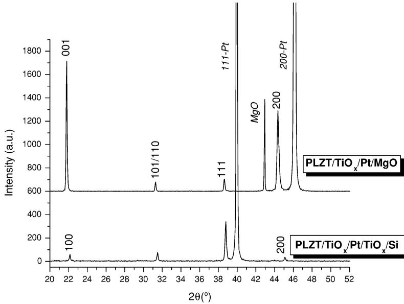
**Figure 2.** X-ray diffraction diagrams of PLZT films deposited on different substrates.
