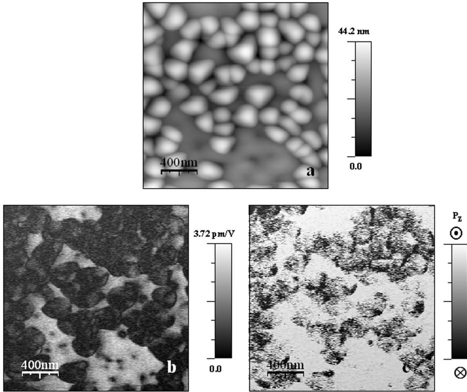
**Figure 5.** SFM images of PLZT films deposited on Ti/Pt/MgO: (a) topography; (b) amplitude and (c) phase of the piezoresponse signal.
