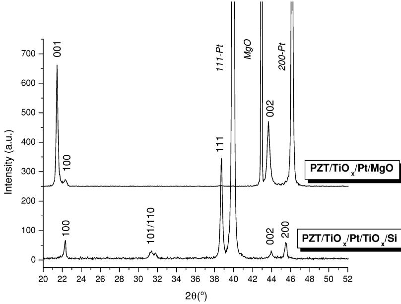
**Figure 1.** X-ray diffraction diagrams of PZT films deposited on different substrates.
