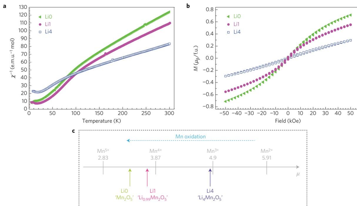
**Figure 4 | Magnetic measurements.** **a**, Susceptibility versus temperature for the as-prepared material  $\text{Li}_4\text{Mn}_2\text{O}_5$  and partially and fully oxidized samples. **b**,  $M(H)$  curves related to these three phases at  $T = 5$  K. **c**, Theoretical and experimental paramagnetic effective moments.
