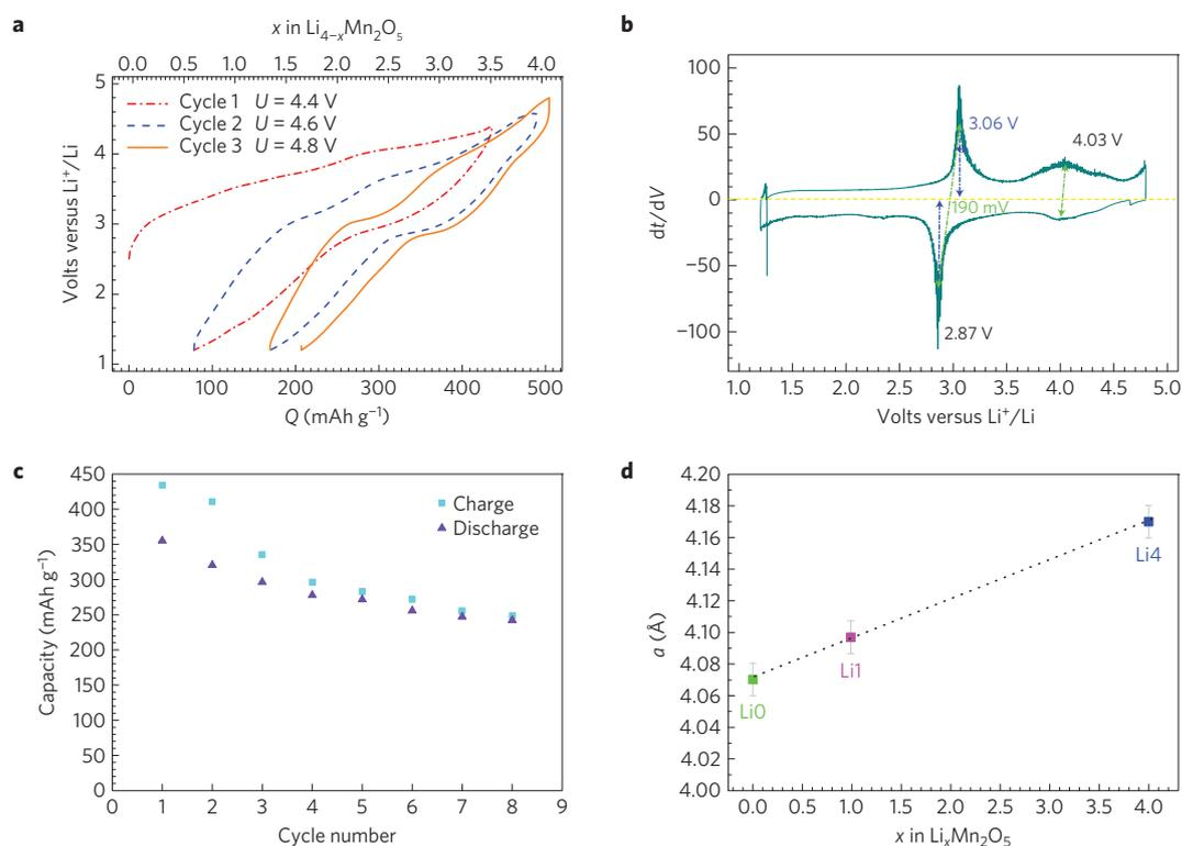
**Figure 3 | Electrochemical properties.** **a**, Typical voltage–composition profile of  $\text{Li}_4\text{Mn}_2\text{O}_5$  obtained at C/20. **b**, Derivative curve  $dt/dV$  versus voltage for the third cycle. **c**, Discharge capacity versus cycle number of  $\text{Li}_4\text{Mn}_2\text{O}_5$ . **d**, Evolution of the cell parameters for the Li4, Li1 and Li0 phases.
