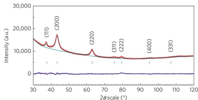
**Figure 1 | XRPD analysis.** Rietveld-refined XRPD pattern of the ' $\text{Li}_4\text{Mn}_2\text{O}_5$ ' sample using the MAUD software:  $\text{GoF} = 1.53$ ;  $R_{\text{wp}} = 1.58\%$ ;  $R_{\text{Bragg}} = 1.23\%$ ;  $R_{\text{expected}} = 1.03\%$ .
