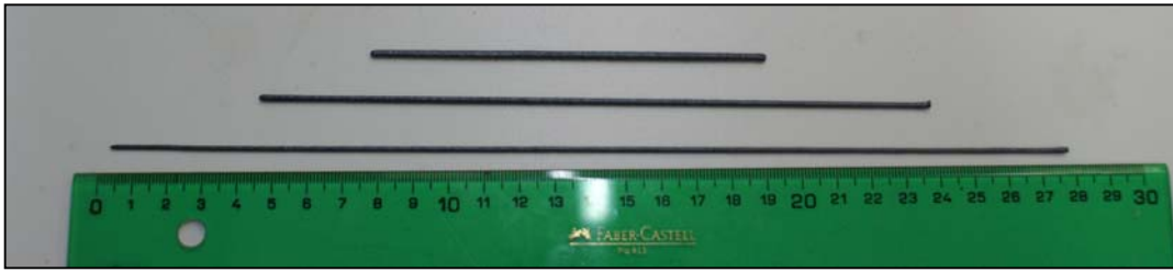
Figure 1: \text{Bi}_2\text{Ca}_2\text{Co}_{1.7}\text{O}_x grown rods depending of their initial green shapes before the translating growth (50 mm/h).
