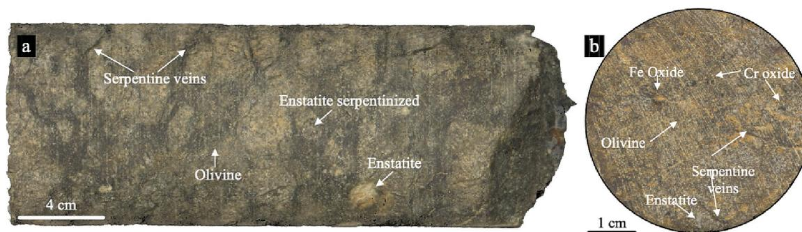
Fig. 1. Macroscopic photographs of the H10 serpentinized harzburgite. (a) Drill core showing olivine matrix, serpentine veins network, enstatite serpentinized and enstatite, and (b) as-sawn sample of the drilled core showing iron oxide, chromite, olivine matrix and serpentine veins network.
