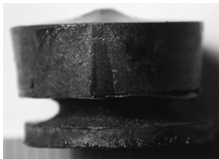
Fig. 2. As-grown bulk sample obtained from ITSG-process showing the strong shrinkage of the source and the single-grain growth along the whole height of the pellet, evidenced by the contrast on the section.
