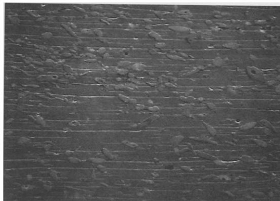
Fig. 3. Typical texture of 123 (sample R102, Table 1). The sample has only one large single domain.
