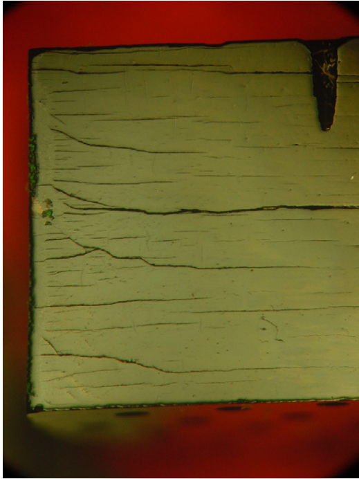
Figure 13. Macrograph using a stereo microscope of an a/c -section taken from a drilled sample (thickness \sim 6 mm) with a classical oxygenation characterized by an intensive cracking along the a/b -planes.
