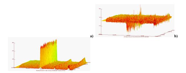
One 2D Debye-Scherrer pattern for one sample orientation without field (left) and difference pattern for the corresponding sample orientation (right).
