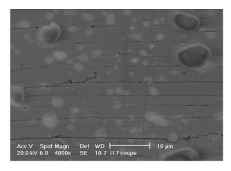
Figure 1: (a) Textured Y123 as-processed and (b) microstructure showing the refined Y211 particles into the Y123 matrix.
