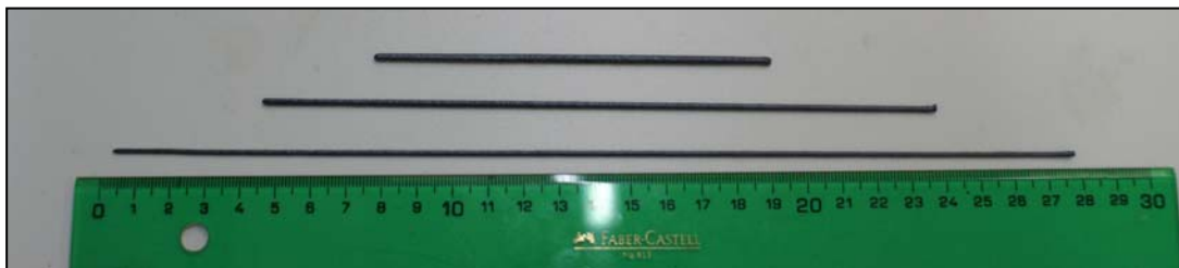
Figure 1: \text{Bi}_2\text{Ca}_2\text{Co}_{1.7}\text{O}_x grown rods depending of their initial green shapes before the translating growth (50 mm/h).
