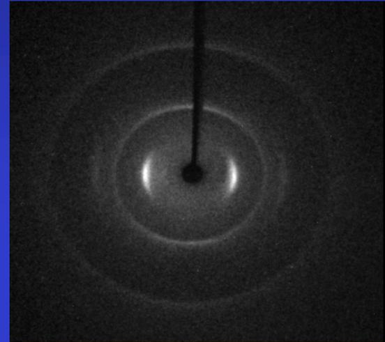
1 fibre (7 microns diameter): CCD Kappa diffractometer
